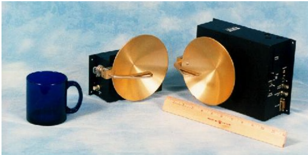
ZDL-111-305, 90.5 GHz Communications System with optional Prime Focus Parabolic
